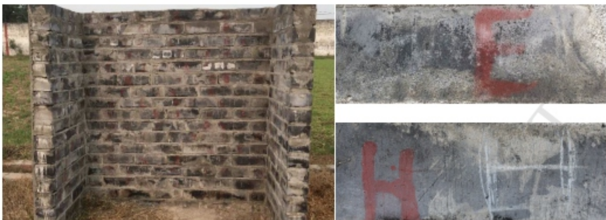
Fig. 24: Biomass ash brick wall subjected to outside environment [155]
