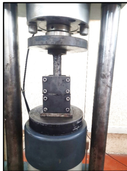
Fig. 31: Setup of the mould used to make biomass ash-based binder cubes
